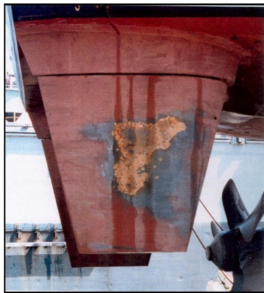
Figure 2: Cavitation erosion of a ship rudder (Shen et al. 1997).
